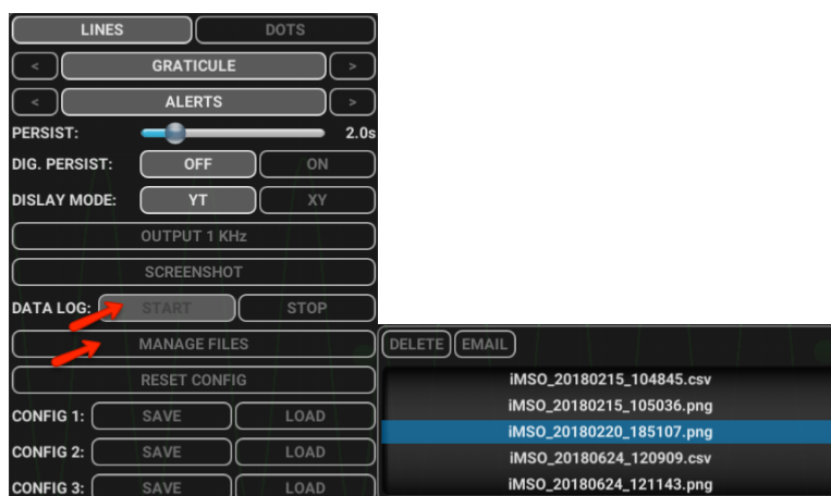
Figure 13: Data logging controls in the iMSO software (L) and pick wheel of captured screenshots and data logs from the manage files menu (R).
